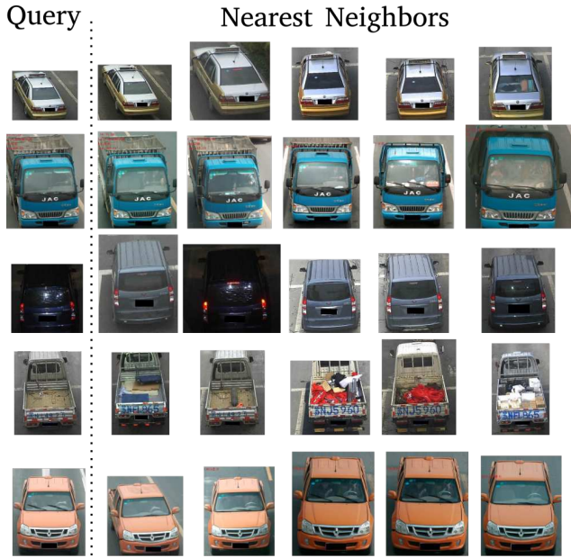
Figure 3: Qualitative image retrieval results on PKU VehicleID [29]. We show 5 nearest neighbors per randomly chosen query image given our trained features. The queries and retrieved images are taken from the test set of the dataset.
